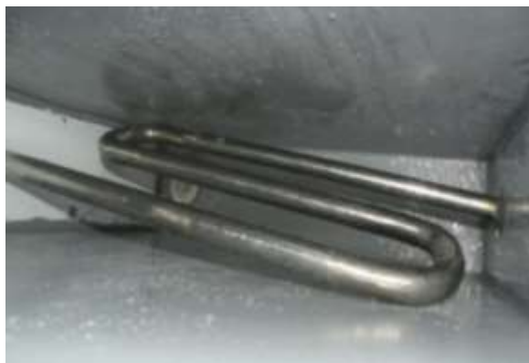
Fig 2.Indirect type partially cold Heat Exchanger
