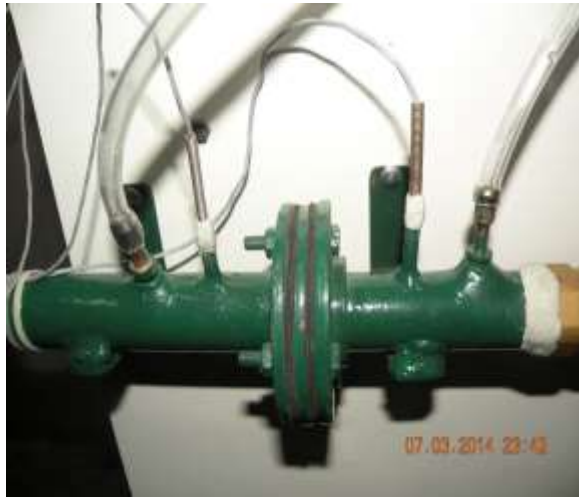
Fig 1.Schematic of orifice meter
